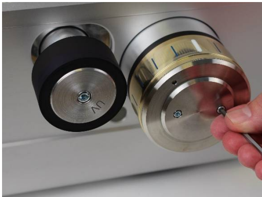
Close cover with two hexagonal screws
