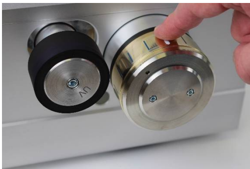
Feel with your finger tip whether the piston is too high, too low or in exact position.
