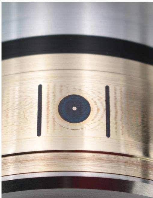
Figure 1 Microwave water content sensor embedded into brass roller
