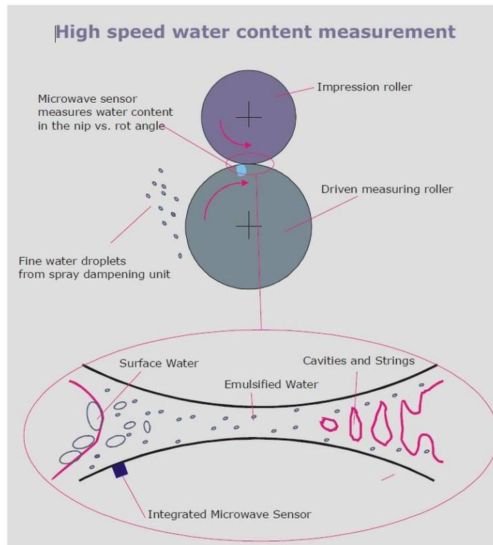
Figure 123 Schematic cross section of nip with emulsion under test
