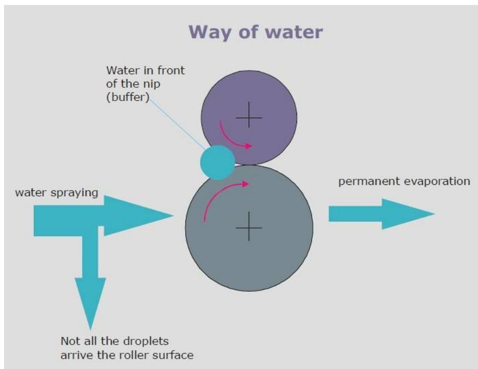
Figure 12 Way of water during a LithoTack II spray cycle
