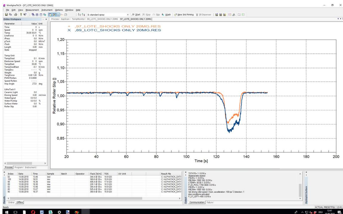
Figure 10 Different viscosity development during water shocks and cycle, ink 97 is essentially more stable unlike ink 89 under presence of water
