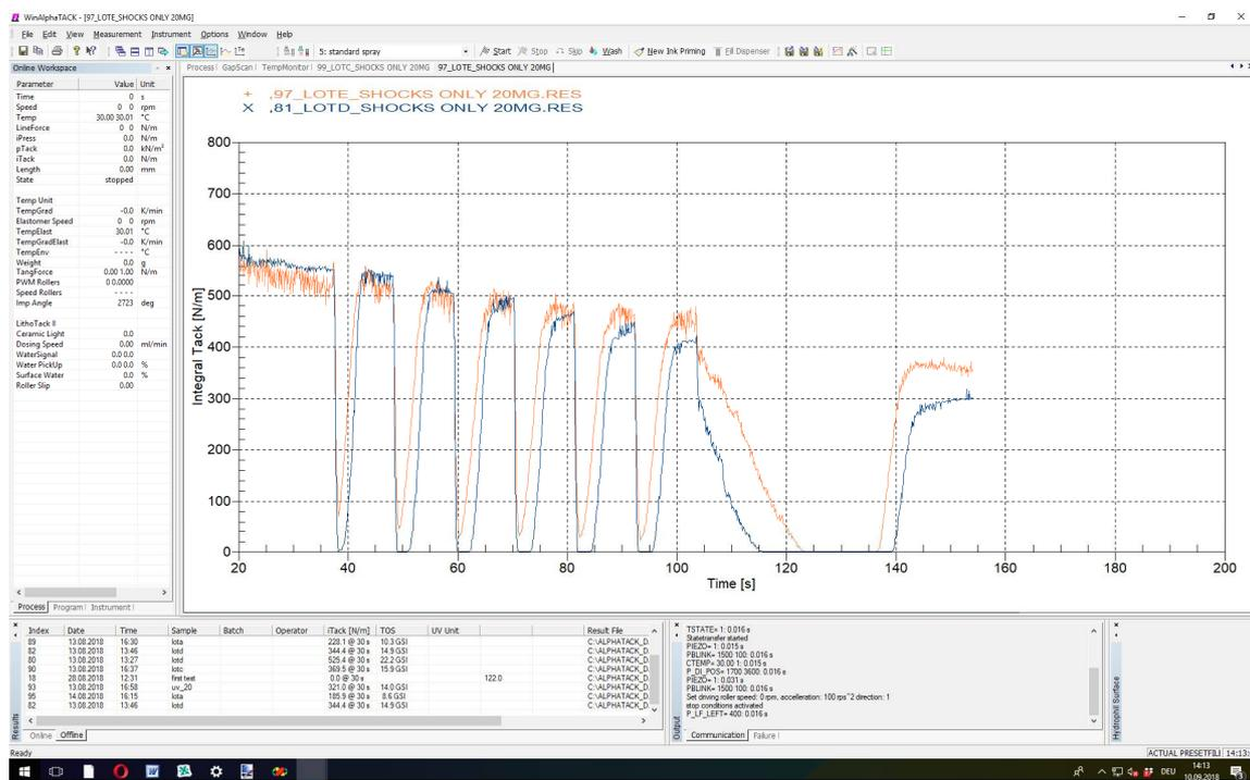
Figure 9 Different tack development during water shocks and cycle, ink 97 is essentially more stable unlike ink 81 under presence of water
