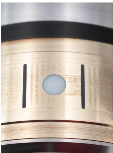
Figure 2 Hydrophil surface spot embedded into brass roller
