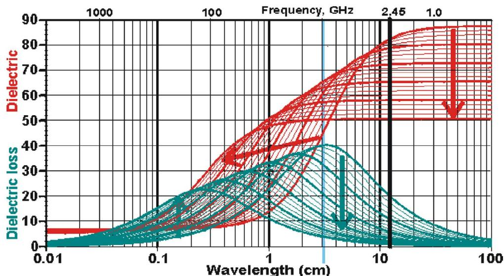
Figure 14 Dielectric permittivity and dielectric loss of water between 0°C and 100°C, the arrows showing the effect of increasing temperature, the blue line indicates the operation point of the LithoTack sensor
