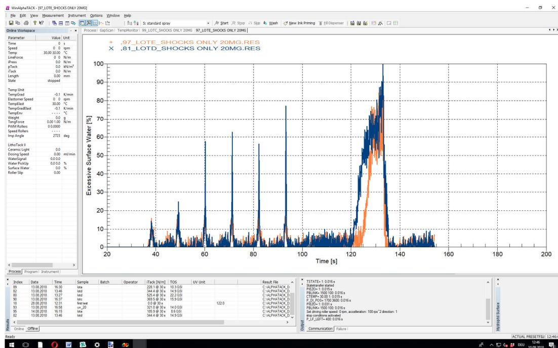
Figure 11 Different amount of excessive surface water during water shocks and cycle, ink 97 shows nearly no surface water when “shocked” compared to ink 89
