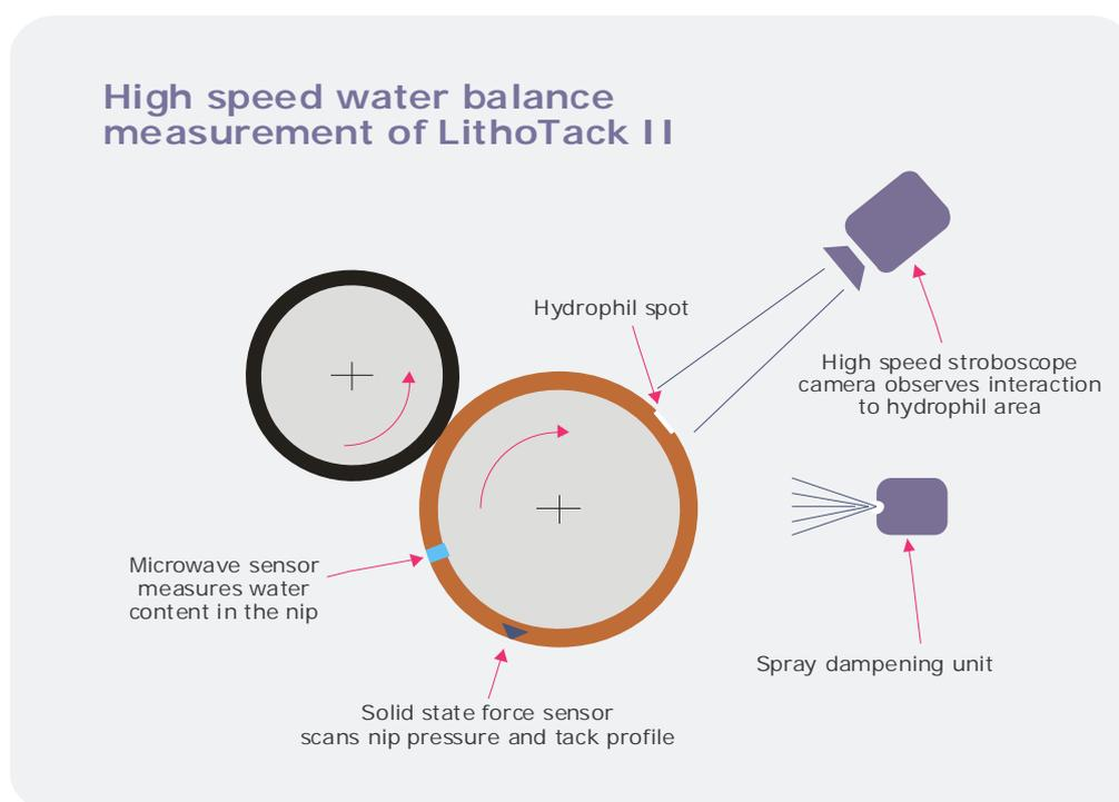
Figure 5 – Principle of high speed water balance measurement
